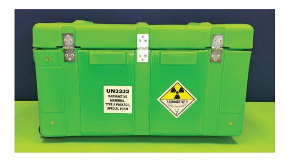
Yellow-II hazard labels, UN Number and proper shipping name on both the hinge side and clasp side of the case.
